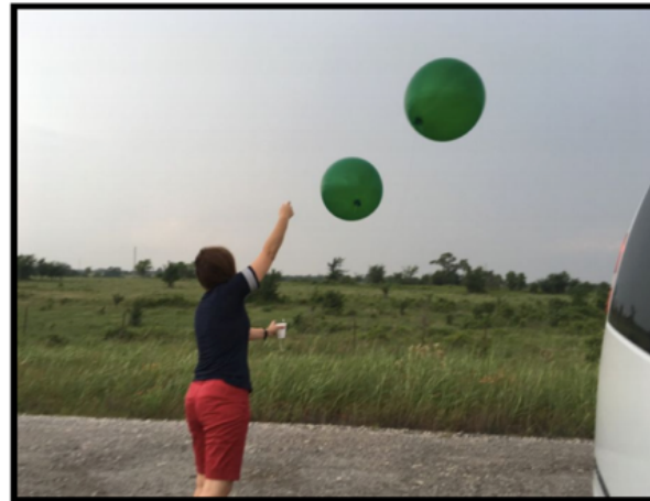
A Swarmsonde is released with two balloons attached to the sonde
